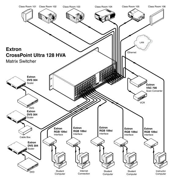
Figure 1-1 — Typical CrossPoint Ultra matrix switcher application
